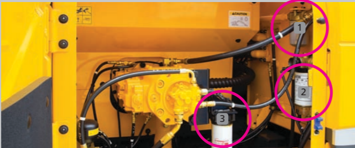
Filter with Extended Exchange Interval (1,000hr)
