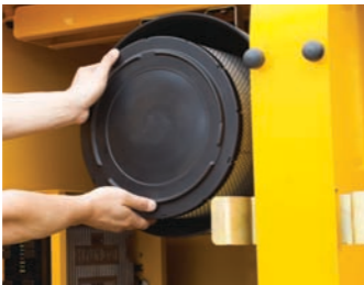
Easy to Change Air Cleaner Assembly
