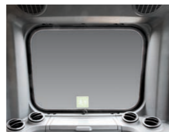
Rear Window Emergency Exit
