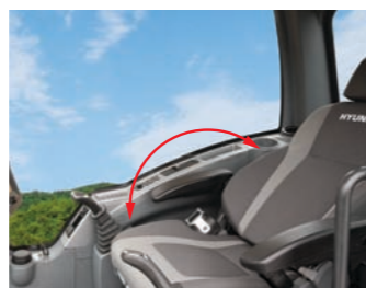
Increased Tilt Angle of Operator's Seat
